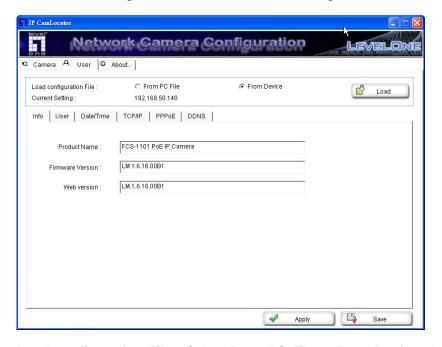
**Load configuration File :** Select **From PC File** or **From Device**, the former can load information of downloaded configuration file and the latter can load Network Camera configurations in the network.
